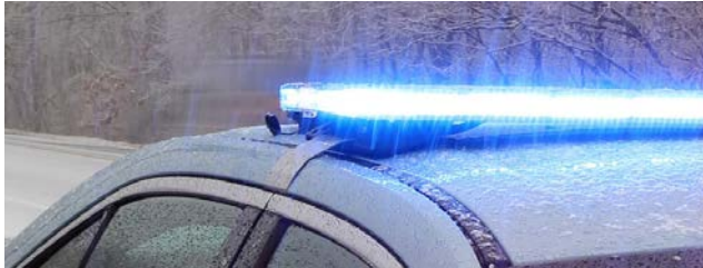
Multi-angled combo corner modules produce light straight out and to critical 45° angles.
